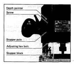
Raise the stopper pole until the desired depth of cut is obtained. The depth of cut is indicated on the scale (1 mm or 1/16" per graduation) by the depth pointer. Then tighten the screw to secure the stopper pole.
